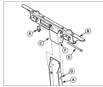
Figure 5. Install Bag and Cover Support
